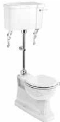
S trap medium level WC with 440 lever cistern W: 440 D: 740 H: 1425 Pan: P18 Lever Cistern: C3 Button Cistern: C4 Flush Pipe: T33 CHR
