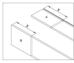
Cut the plumbing cover based on the dimension X.
