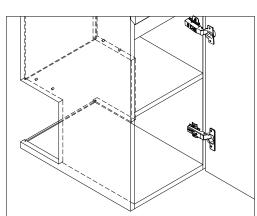
Insert the plastic bolts into the 4 holes on both sides.
