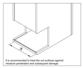
Cut off the plumbing section as per the marked lines. Measure the inner dimension "X" of the unit as show in the above diagram.
