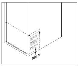
Following the template mark out the cutting lines. If necessary, please use a spirit level.
