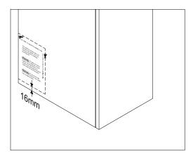
Attach the template supplied with the plumbing cover to the unit.
