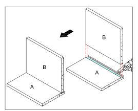
Please apply silicon to the slot in board A, and then fit board B into A properly.
