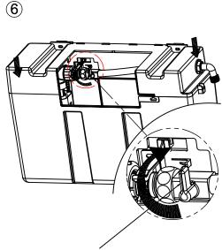
Adjust the flexible pipe to make sure the insulating valve is facing the front of the tank.
