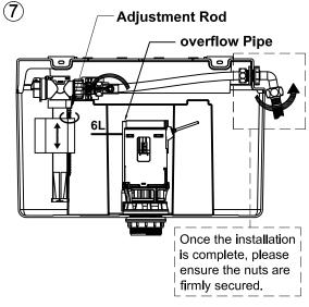
Connect the water supply to the inlet elbow and turn on the insulating valve.
