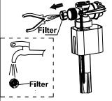
Pull out the filter from the Inlet. Clean by rinsing the filter.
