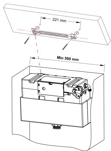
2. Note the minimum width required for this cistern is 560mm.
