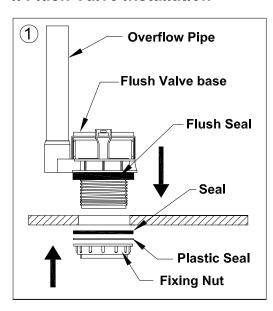
Insert flush valve base and flush seal through the tank flush hole. Tighten with the fixing nut, clamping the seals in place.
