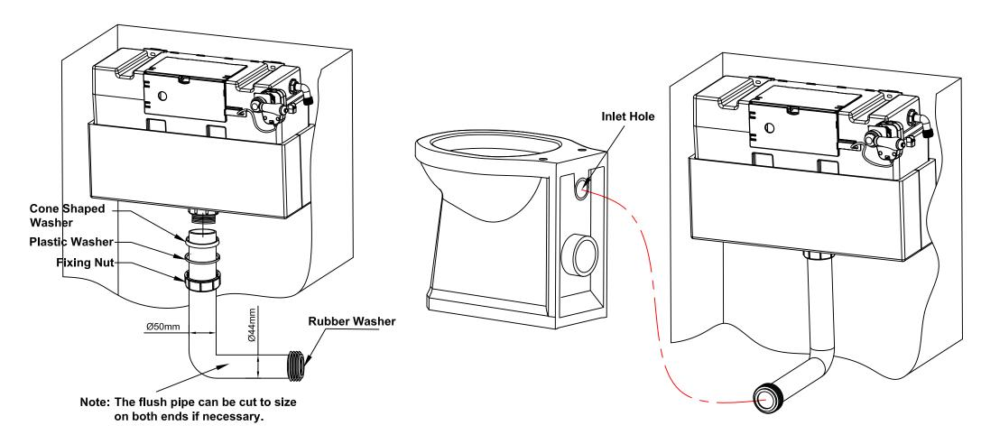
3. Place the fixing nut, plastic washer and cone shaped washer onto the end of the flush pipe with diameter 50mm.
