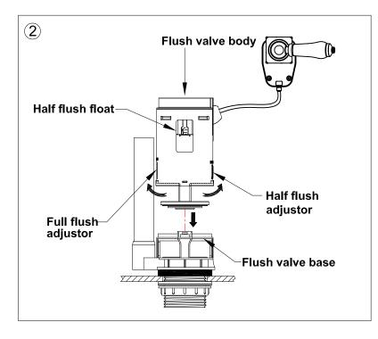
Insert flush valve body into the flush valve base, rotating it until it fixes onto the clip.
