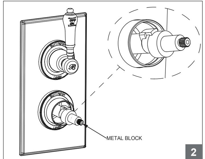
1 ) Remove the temperature control handle, metal block as the page 2 diagram.
