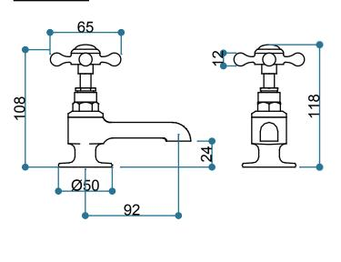
Identify the hot tap and position into the basin on the left hand side, from the underside of the basin fit the rubber washer and then the nut. Making sure the tap is in the right position tighten the nut to secure the tap to the basin.
