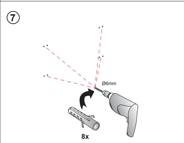
Drill holes using the Ø6mm drill bit following the marked positions, and insert the wall plugs.
