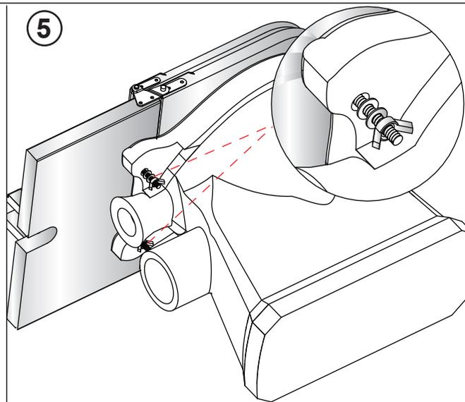
Reposition the seat with the fixing bolt inserted into the pan holes. Ensure the position is fit, and fix onto the pan by sliding up the rubber washer, brass washer and finally tighten by the nut.
