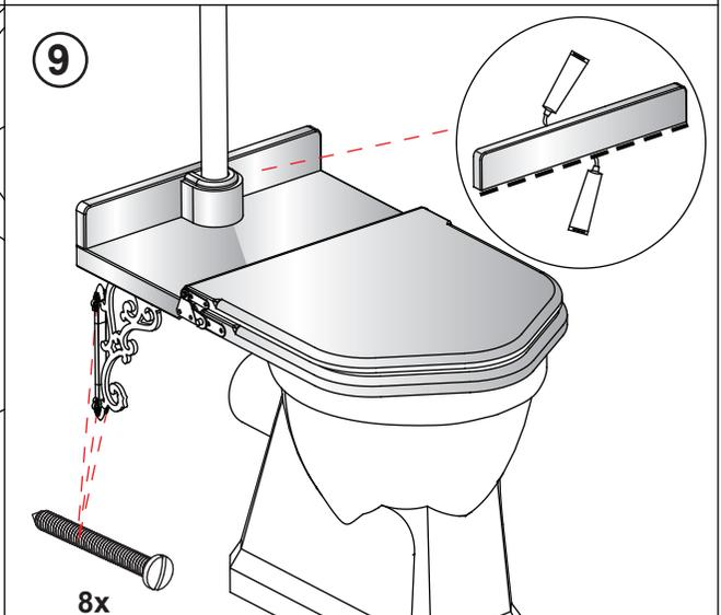
Reposition the seat against the wall, align the ornate bracket holes with the predrilled holes on the wall, fix onto the wall by tightening the screw supplied. Finally attach the back board to the wall and seat using a suitable mastic for use with wood and tiled surfaces.
