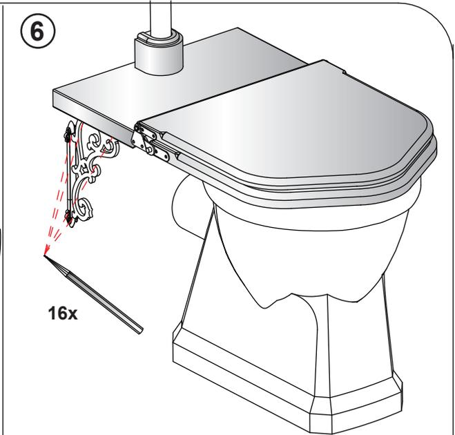
Place the ornate bracket into the fit position. Mark the fixing hole positions onto the wall and the seat by pencil.
