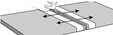
14. Once cured, the bead of adhesive can be removed by sanding with a random orbital sander with the following order of sandpaper grades: P120 to remove the adhesive bead, P240, P320, P500 grit and then finish with a grey abrasive pad and a light mist of water. All stages must be carried out with the random orbital sander.
