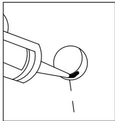
Once the bath is in the general position ready to be plumbed in, we suggest fitting the waste and overflow to the bath. Before you do this we insist you smear silicone sealant around the inside of the overflow and waste to ensure a totally water tight seal. This is shown in the diagram above.
