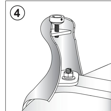
To secure the bath to the floor place a small amount of silicone under each foot where it meets the floor.
