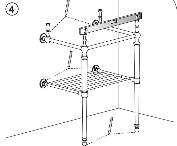
4 Place the basin stand with shelf onto the wall, use a pencil to mark the screw holes on the wall and floor.
