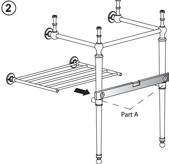
2 Assemble the shelf with part A as shown in above diagram.
