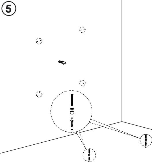
5 Use a drill bit to drill holes.
