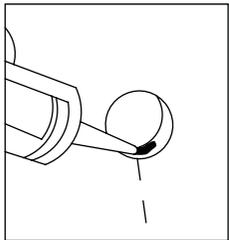
Once the bath is in the general position ready to be plumbed in, we suggest fitting the waste and overflow to the bath. Before you do this Burlington insists you smear silicone sealant around the inside of the overflow and waste to ensure a totally water tight seal. This is shown in the diagram above.
