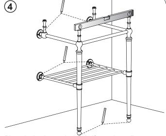
Place the basin stand with shelf onto the wall, use a pencil to mark the screw holes on the wall and floor.
