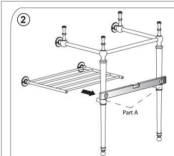
Assemble the shelf with part A as shown in above diagram.
