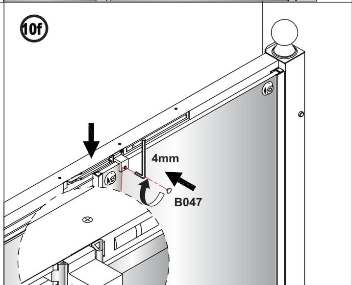
Make sure the door is closed well and there are no gaps. As indicated in the diagram between the clasps of the mechanism place the catch over the glass, and tighten to glass.
