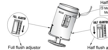
2 Move adjustor down, flush volume increases. Move float up, flush volume decreases.
