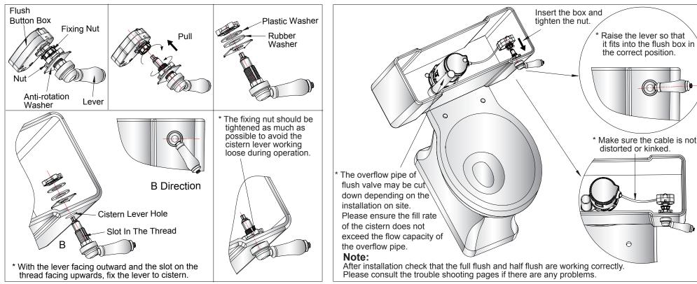
\* Make sure the cable is not distorted or kinked. 0 After installation check that the full flush and half flush are working correctly. Please consult the trouble shooting pages if there are any problems.
