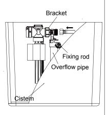
Fix the inlet valve onto the overflow pipe, and tighten the fixing rod.
