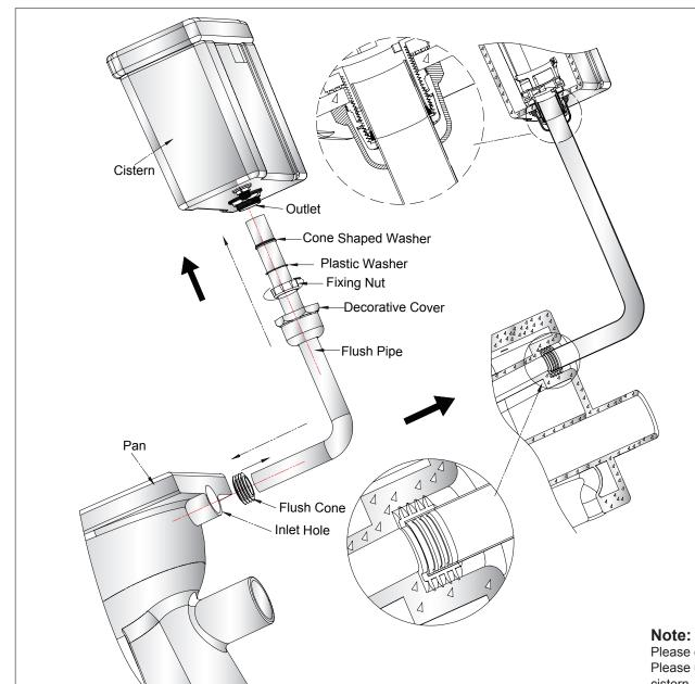
Determine the exact location of the pan and cistern installation, then cut the Flush Pipe accordingly if necessary. Fit the Pipe into the cistern in the sequence shown in the diagram.
