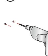
Using a 6mm drill bit, drill holes in the marked positions.
