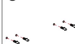
Insert the rawl plugs into the drilled holes.
