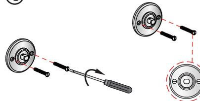
Screw in the stainless steel screws to secure the base to the wall.
