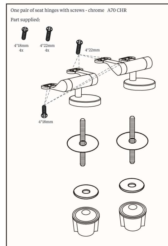
Uninstall the soft close hinges pre-fitted on the seat and install the chrome ones. Please reference the instruction supplied with the product for the detailed fitting steps.
