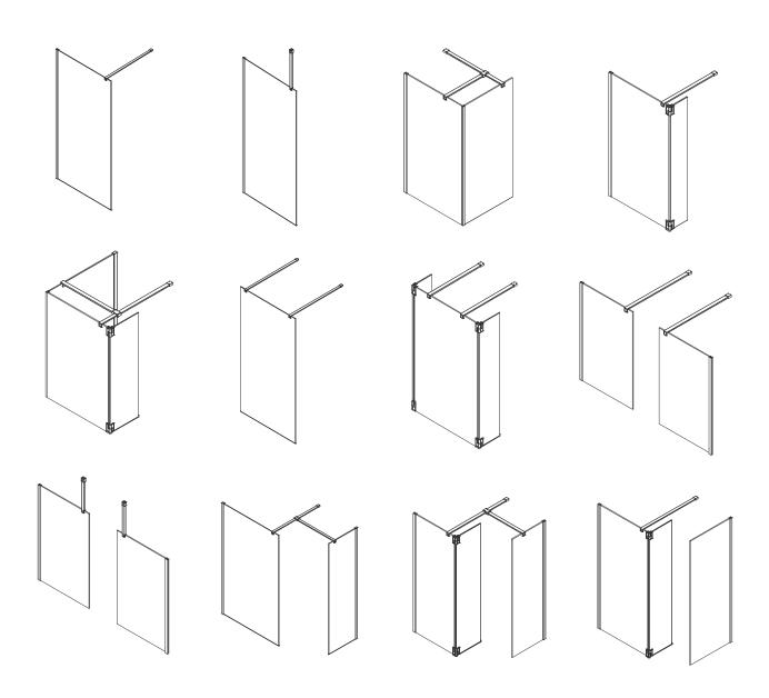
We recommend the entry width the above configurations is a minimum of  $500\,\mathrm{mm}$
