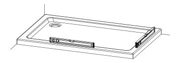
If fitting a tray we recommend a drainage test is carried out before the tray is tiled in position.
