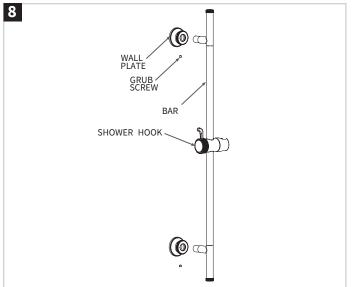
Make sure the shower hook at a suitable position. Insert and fix the bar to the wall plates with grub screws.
