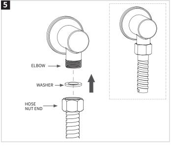
Connect the elbow with the outlet.
