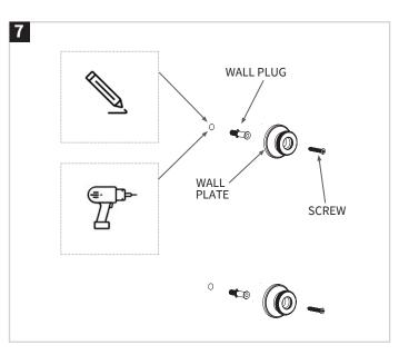
Make sure all is right, mark out the two fixing hole positions on wall. Drill holes. Insert wall plugs. Fix the wall plates onto the wall by screws.
