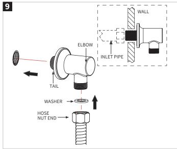
Connect the elbow with the outlet. Connect the hose nut end with the elbow .
