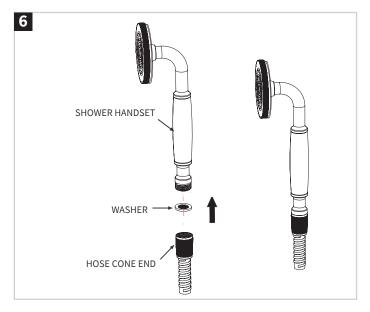
Connect the hose cone end and washer with the shower handset.
