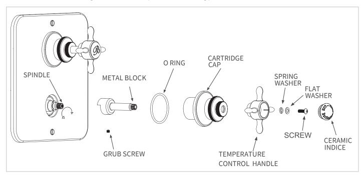
Pick off the ceramic indice and loosen the screw.
