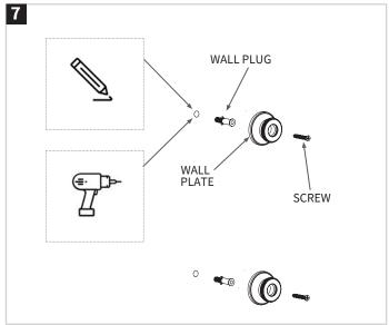
Make sure all is right, mark out the two fixing hole positions on wall. Drill holes. Insert wall plugs. Fix the wall plates onto the wall by screws.
