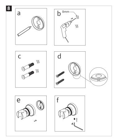
a) Measure and mark the desired location and ensure the mounting bracket is aligned correctly. Use the mounting bracket as a template to mark the drill holes on the wall.
