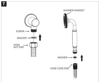
Connect the hose nut end and washer with the elbow. Connect the hose cone end and washer with the shower handset.
