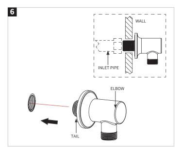
Connect the elbow with the outlet.
