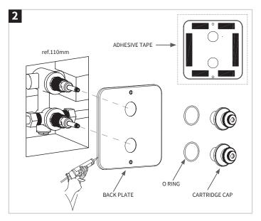
Mount the O-rings and cartridge caps onto the back plate. Make sure the O-rings are stuck in the groove at the bottom of the cartridge caps. Remove the adhesive tape film on the backside of back plate. Tighten cartridge caps onto the cartridge, and paste the back plate on the wall. Apply a narrow bead of silicone sealant around the back edge of the back plate and carefully press into position.
