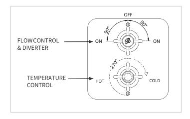
1. Turn the flow control & diverter handle to increase/ decrease the water flow and switch the outlet.
