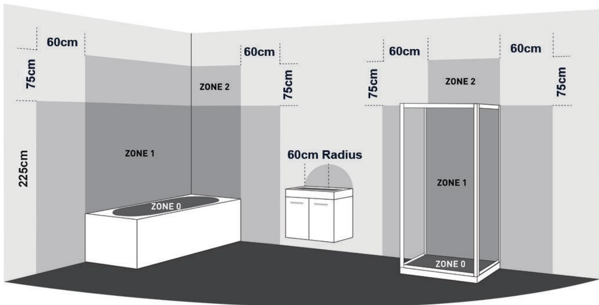
This product is IP44 rated and is suitable for installation within zone 2 above, and complies with the following safety standards: EN 60598
