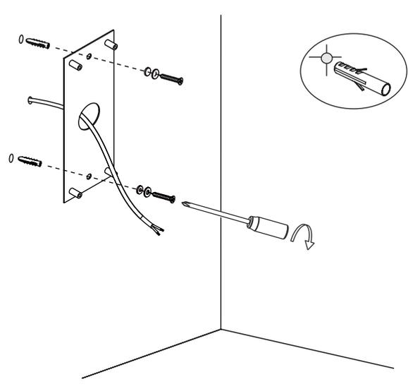
Insert the wall plugs into the holes drilled and secure the wall bracket to the wall with screws provided. Pull the wiring through the hole and secure the bracket to the wall ensuring it is fully flush.
