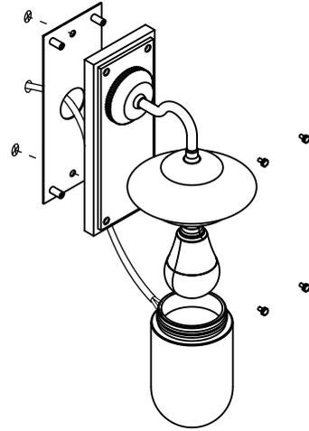
Remove the 4 screws on the front of the light by hand, to release the wall bracket from the assembly. Carefully put aside the light assembly to begin installation.
