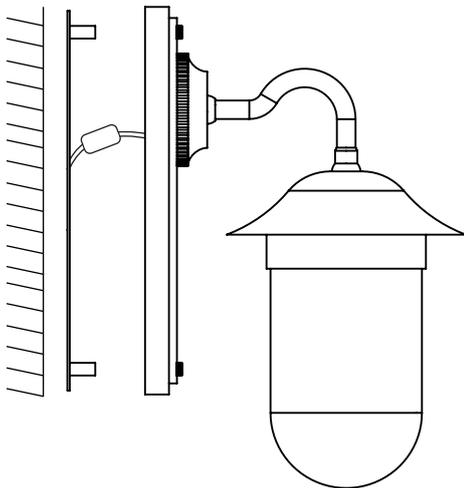
Align the light to the wall bracket and ensure the electrical wire is not trapped. Tighten the screw fixings on either side of the base.
