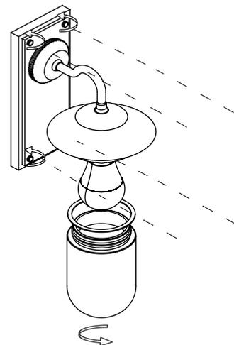
Secure the light to the wall bracket by hand tightening the textured, decorative screws. Fix the bulb to the light and screw the light cover into position. Ensure the silicone ring is present and correctly fitted on the glass shoulder as this component ensures the seal for IP44.
