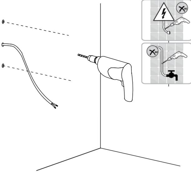
Determine the installation position of the light and mark the wall through the screw holes on the inside of the wall bracket, ensuring they are level.
