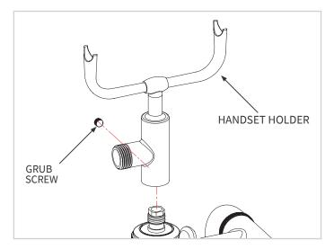
Loosen the grub screw on the handset holder by using the allen key and insert the bath shower mixer connector into the handset holder, then tight the grub screw back to the holder.
