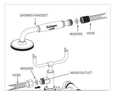
Insert a washer into the nut end of hose and tighten it to the mixer outlet. Insert another washer into the cone end of hose and tight it with shower handset.
