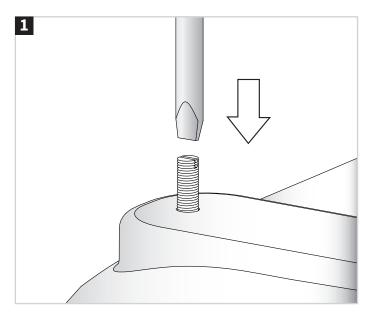
With the bath safely placed upside down, locate the threaded fixing bolt onto the fixing points on the underside of the bath.
