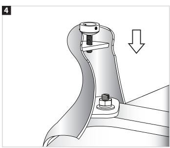
Locate the adjustable feet on the bottom of the bath legs. Repeat steps 1 to 4 for all bath legs.
