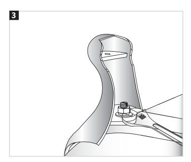
Tighten the nut using an adjustable spanner, securing the leg to the bath with a tight fit.
