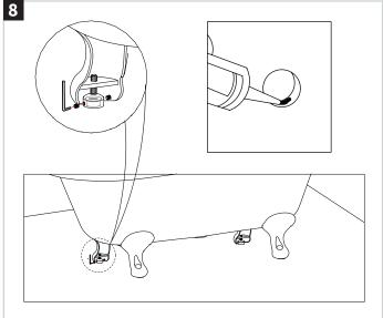
Lock the bath feet in place using the allen key and grub screws provided. Once the bath is in the general position ready to be plumbed in, we suggest fitting the waste and overflow to the bath. Before you do this Burlington insists you smear silicone sealant around the inside of the overflow and waste to ensure a totally water tight seal. This is shown in the diagram above.
