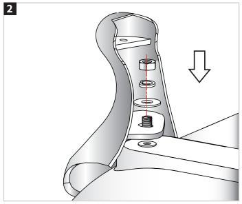
Assemble the fixing nuts and washers as shown in the diagram. Extra washers are included to provide additional adjustment for the mating of the leg to the bath if required.
