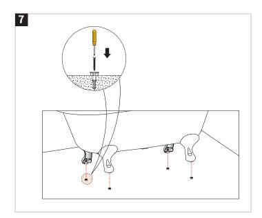
Secure the bath feet locators to the floor with a Phillips screw driver. Locate the bath onto the bath feet and once again, check to ensure the bath is level.
