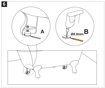
With the bath adjusted to be level and placed in the desired location, mark the position of all 4 feet. Drill the holes centrally making sure to use the correct fixings for the floor structure.
