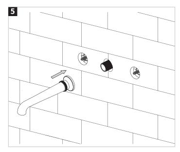
Screw the spout onto the connector. Adjust the spout so that the outlet is facing down.
