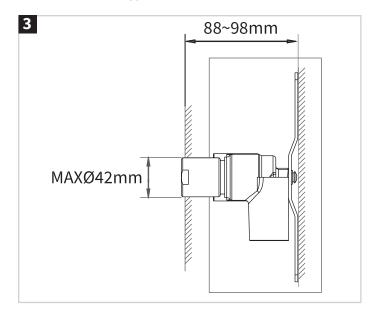
Tile the wall, The thickness should be fixed between 88 to 98 mm from the tile to the bottom of the bracket.
