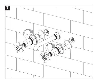
Screw the collars onto valve body.
