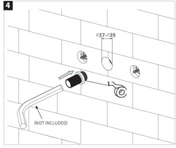
Seal the connector and fully screw onto the valve body on the wall.
