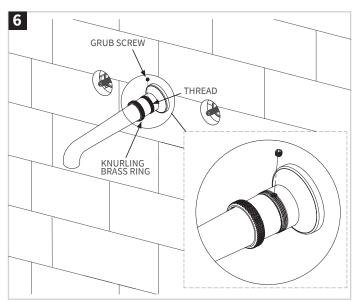
Loosen the knurling brass ring until the thread and grub screw are visible, and tighten the grub screw. Do not damage the surface of the spout. Tighten the knurling brass ring back in place.
