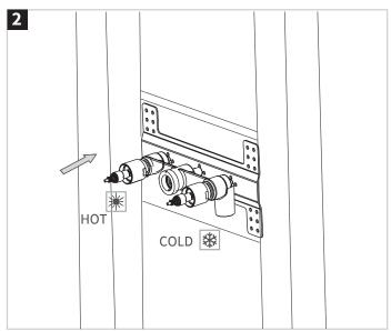
Connect the hot (to the left) and cold (to the right) water supplies to the 1/2 fixing at the bottom of valve body. Please note the tile should be fixed between the MAX marking and MIN marking on the protective covers.
