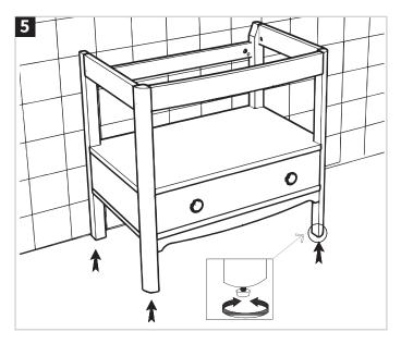
Ensure the cabinet is straight and level by adjusting the feet at the bottom of the furniture legs.
