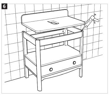
The basin or worktop, tap and waste fittings may now be installed, following the manufacturer's instructions. Connect water and waste pipework and turn on the water supply to check for any leaks.
