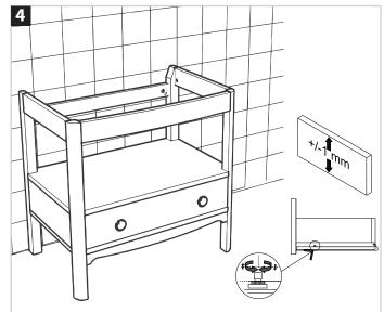
Install the wall brackets using the fixings provided. The unit carcass can now be mounted on the wall brackets and adjusted to ensure it is flush with the wall and level.
