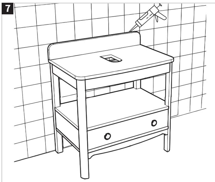
Apply silicone sealant at the back and top of the basin and unit to keep watertight. Check the manufacturer's instructions for drying times.
