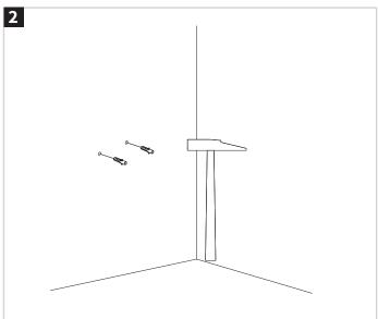
Place wall plug in hole and use hammer lightly to ensure fully in the wall.
