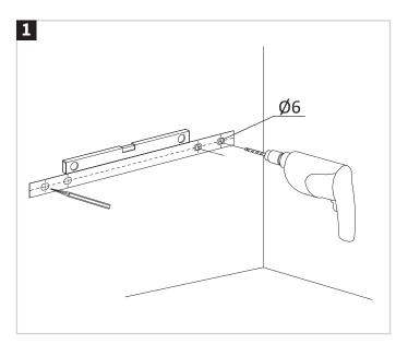
Measure area where accessory will be installed, if there are 2 installation points ensure the holes are straight with a spirit level. Use drill to create hole.
