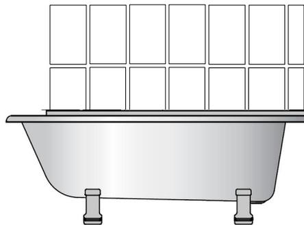
**Tiling the whole wall** The bath should be placed in a position and the wall marked up with the bath rim position. Remove the bath and tile the under bath area. Complete the rest of the tiling except for the first row of tiles above the bath. Fit the bath and then complete the tiling.
