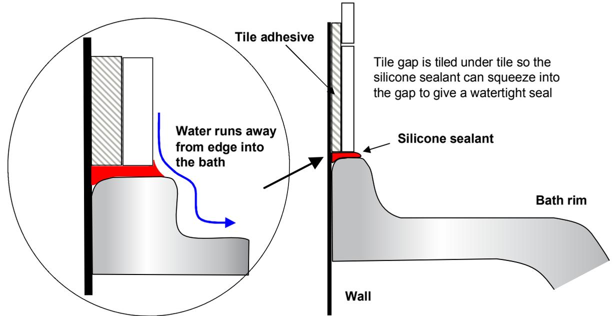
**Tiling the wall above the bath** Plan the tiling to end neatly on top of the upstand
