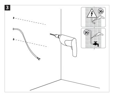
Determine the installation position of the light and mark the wall through the screw holed on the inside of the wall bracket, ensuring they are level.
