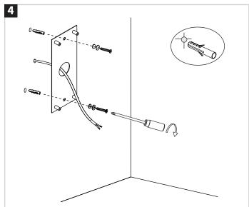
Insert the wall plugs into the holes drilled and secure the wall bracket to the wall with screws provided. Pull the wiring through the hole and secure the bracket to the wall ensuring it is fully flush.
