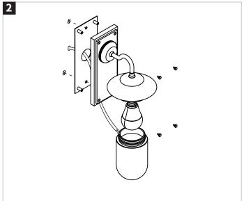
Remove the 4 screws on the front of the light by hand, to release the wall bracket from the assembly.
