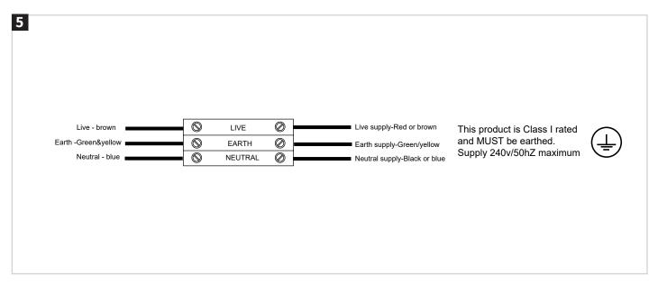
Remove the cover from the electrical connections box. Using a suitable terminal screwdriver make secure connections as follows:
