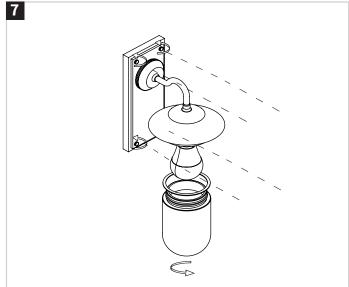
Secure the light to the wall bracket by hand tightening the textured, decorative screws. Fix the bulb to the light and screw the light cover into position. Ensure the silicone ring is present and correclty fitted on the glass shoulder as this component ensures the seal for IP44.
