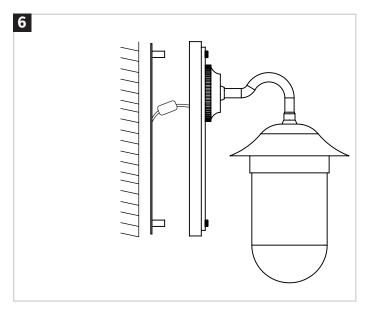
Align the light to the wall bracket and ensure the electrical wire is not trapped. Tighten the screw fixings on either side of the base.
