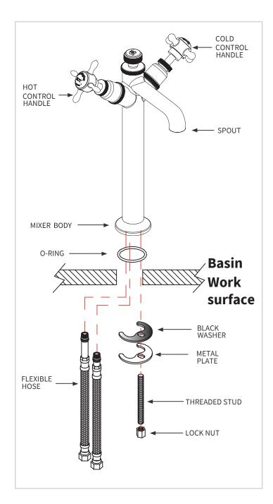
Screw the flexible hoses and threaded stud into the mixer body, and fully hand tighten. Place mixer in position to see if any alteration to the existing supply pipework is necessary.
