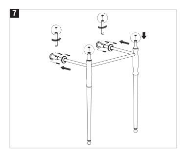
Fix each of the two brackets onto the wall using the 6 screws provided. Ensure that the screw heads are parallel to the floor. Place the 4 rubber washers into the 4 recesses as shown. The 4 rubber washers are not recommended to use when installing the marble basin onto the stand.
