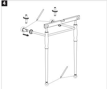
Determine the final installation position and mark the 6 wall and two floor fixing hole positions in pencil. Please make sure to include the floor nipples (and washers if necessary) when determine the installation position because the stand may elevate after the floor nipples are fitted.
