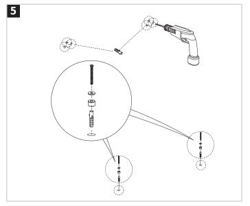
Using a 1/4" drill bit drill the eight holes on the marked positions.
