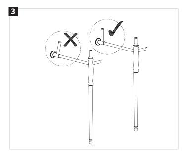
Check that the horizontal bracket bar is vertical using a spirit level.
