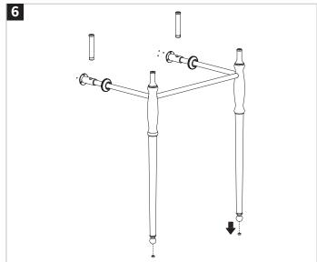
Fit the two legs over the floor nipples.
