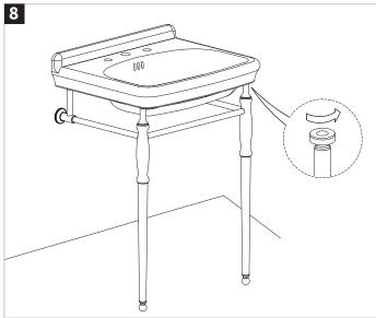
For ceramic basin, place the basin in position ensuring that it is level. The basin must be fixed to the wall at the rear using appropriate wall fixing screws. The top part of the rail can be adjusted slightly if the basin is not level.
