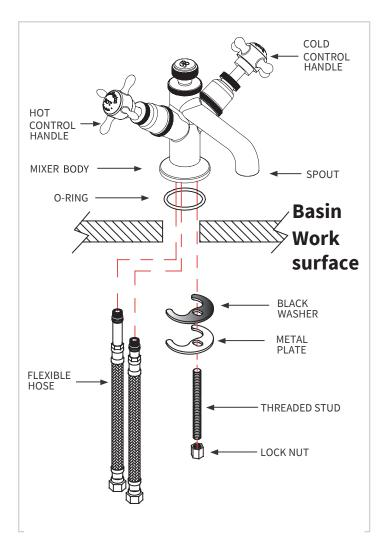
Screw the flexible hoses and threaded stud into the mixer body, and fully hand tighten. Place mixer in position to see if any alteration to the existing supply pipework is necessary.
