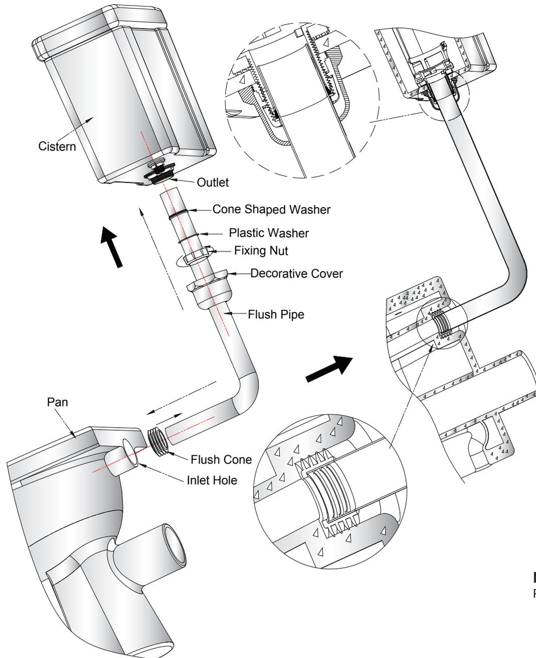
Determine the exact location of the pan and cistern installation, then cut the Flush Pipe accordingly. Fit the Pipe into the cistern in the sequence shown in the diagram. Then insert the Flush Cone into the pan, followed by the Flush Pipe as shown in the diagram.
